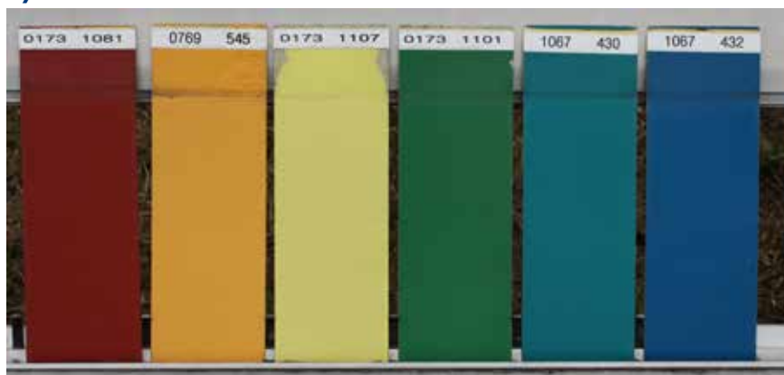
> 40 year Florida Test Fence exposure of Kynar 500® architectural finishes
